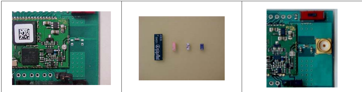
Figure 3. Antenna on PCB Figure 4. Antenna examples Figure 5. SMA connector for external antenna
